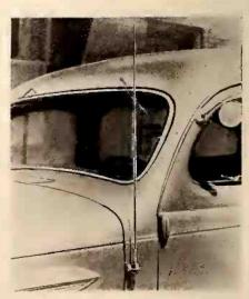
Cowl antenna for older type cars requires no drilling through body. Unit shown is made by Philco.
